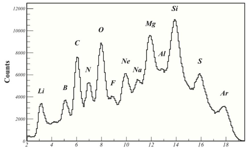
Ar-beam on PSD: Charge spectrum
