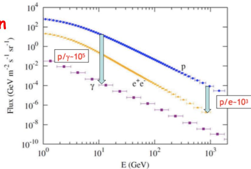
Detection of electrons and gamma-rays
