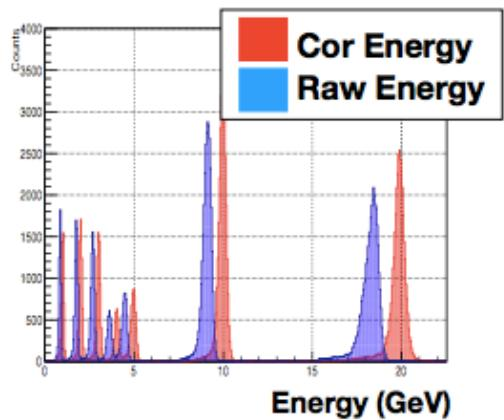
Electron BGO-energy before and after correction
