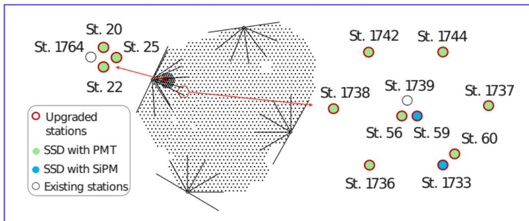
Engineering Array comprising 12 AugerPrime detectors operational since Oct 2016.
