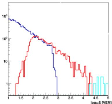
Logarithm of charge for single station measured by standard PMT (blue) and SPMT (red -unsaturated, cyan-saturated).
