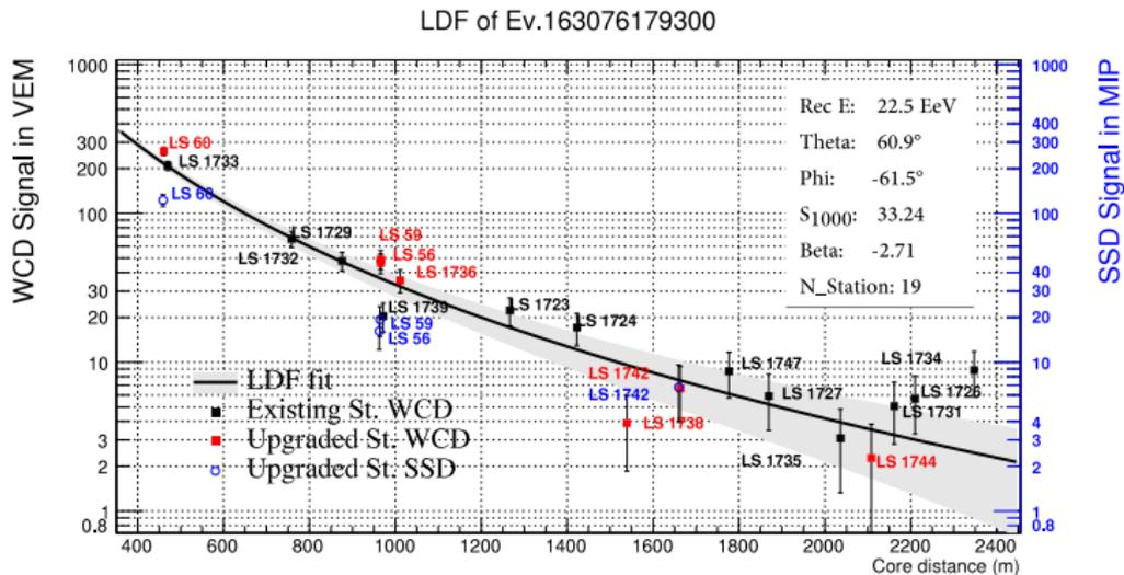
Signals in upgraded local stations (LS) from one event compared with its LDF reconstructed with regular 1500 m array.
