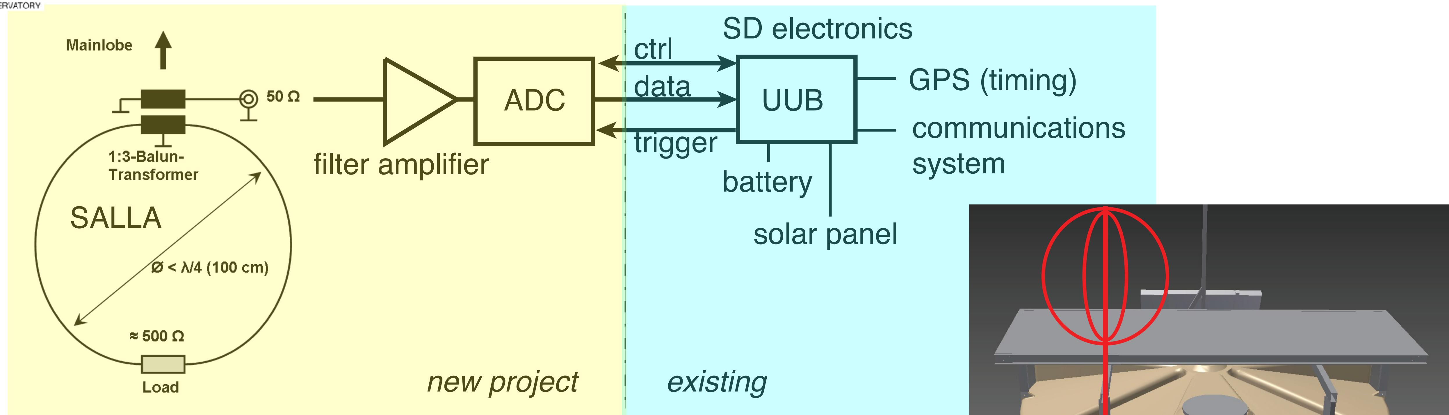
**Shared infrastructure (solar power, battery, GPS timing, communications system) and integrated data acquisition**
