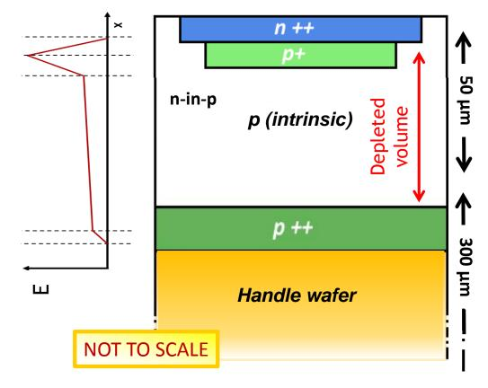
Thin p+ gain layer implanted under the n++ cathode;
