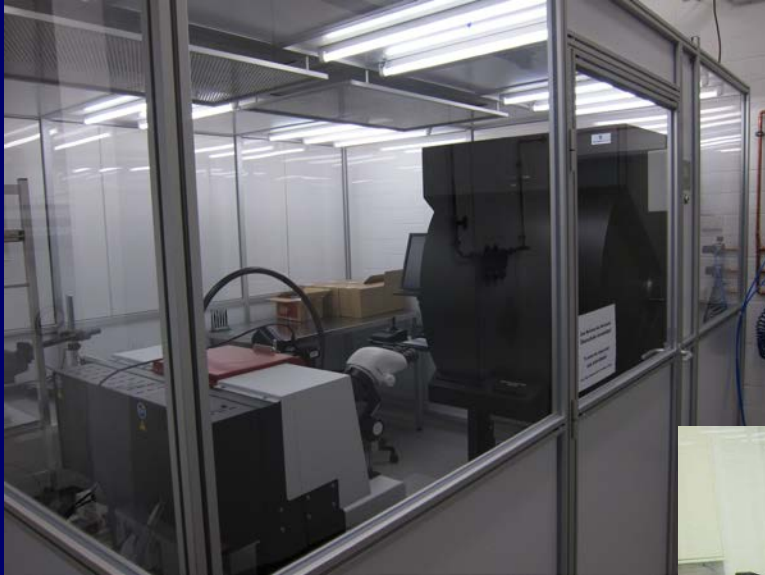
Cleanroom facility (ISO class 6)
