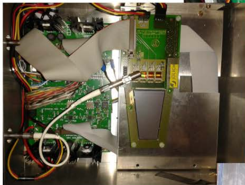
Full-size trapezoidal sensor module (fw disc strips)
