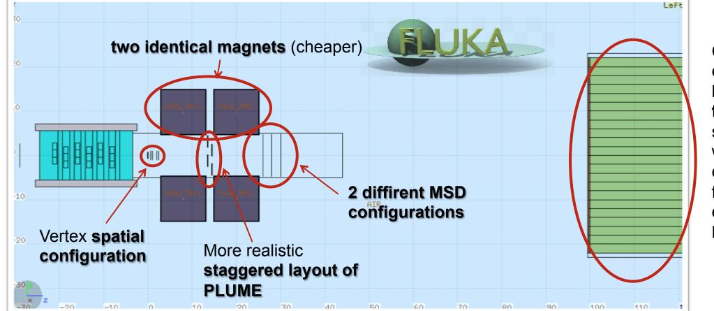
Calorimeter BGO crystals have been **lengthened from 14 to 21 cm** since, hopefully, we will inherit ~21 cm long crystals from L3 experiment at LEP
