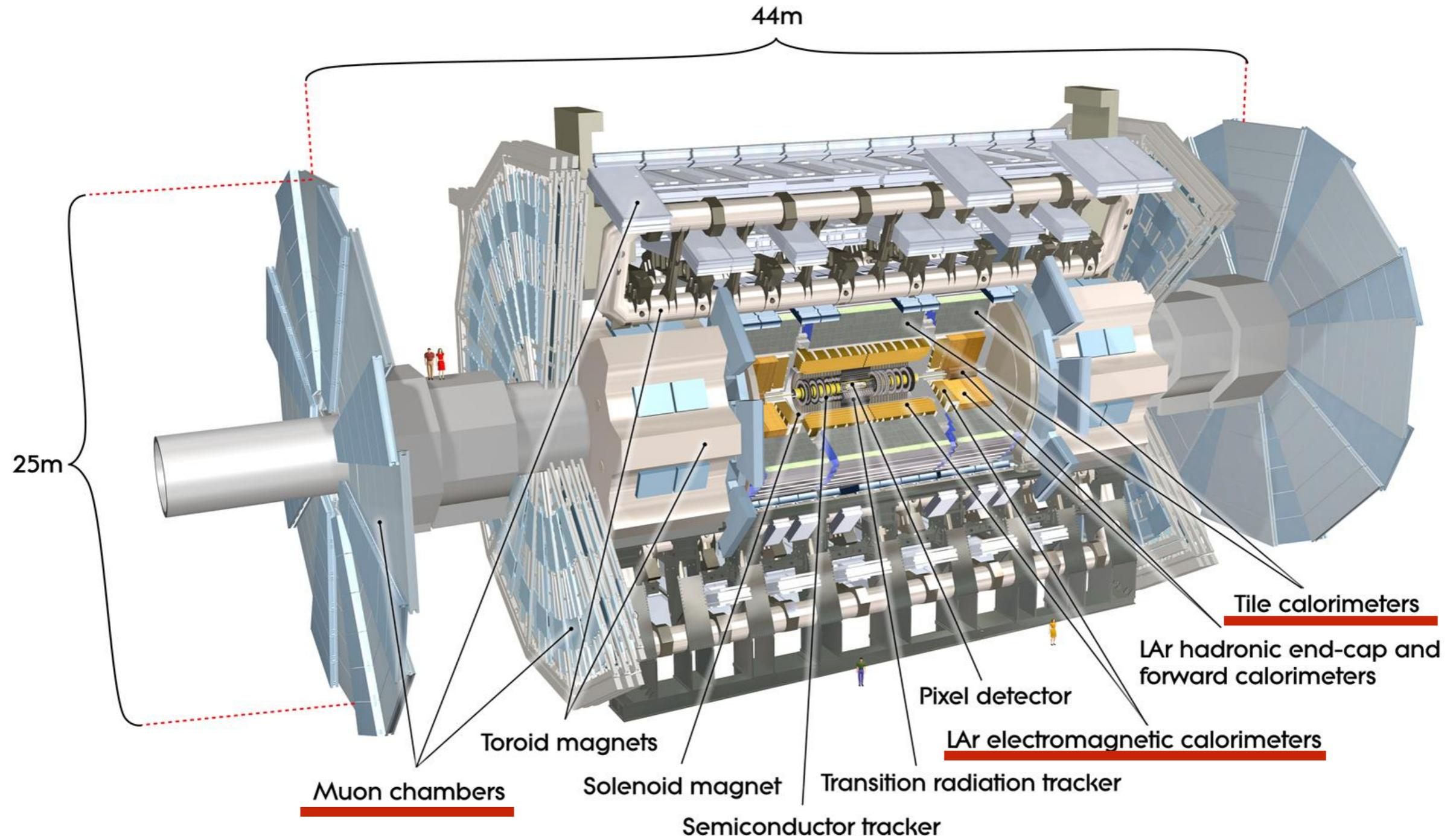
This search will exploit the Muon Spectrometer (MS), the electromagnetic (ECAL) and hadronic calorimeter (HCAL)
