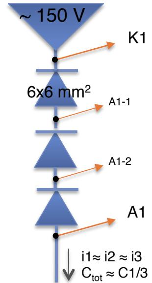
**150 sensors:**  $3 \times 50$  Mu2e pre-production SiPMs from **Hamamatsu**, **SenSI** and **AdvanSiD**
