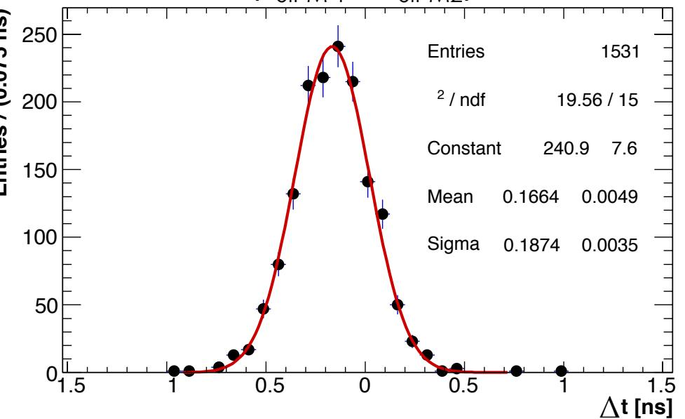
$\sigma(T_1+T_2)/2 \sim 94 \text{ ps}$
