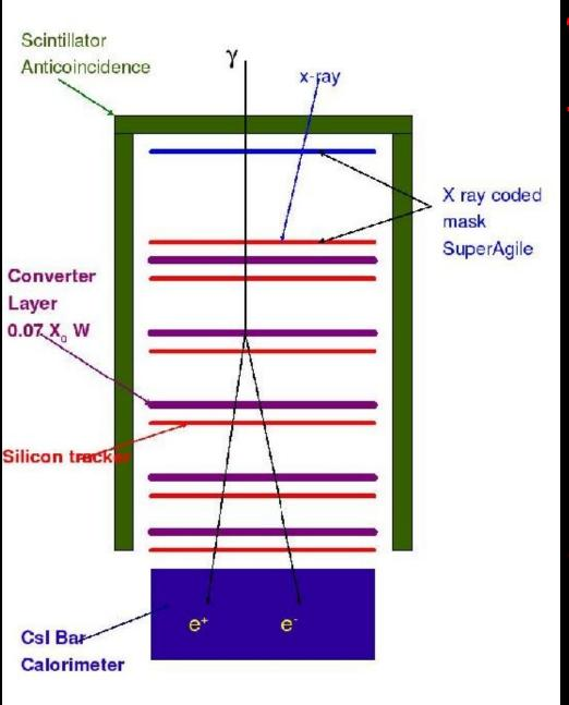
γ-rays detected through pair conversion (e<sup>+</sup>e-) then measured in the Silicon Tracker
