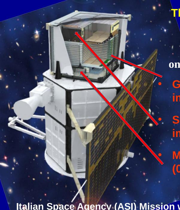
The AGILE Payload: the most compact instrument for HE astrophysics only ~100 kg (~ 60 × 60 cm)
