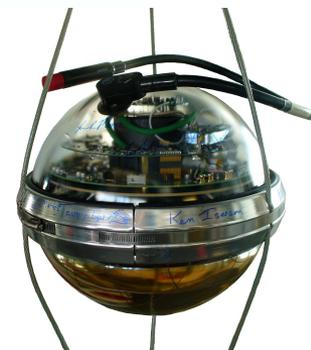
Its main component is a large area hemispherical photomultiplier glued in a pressure resistant glass sphere with optical gel.
