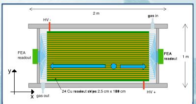
x coordinate: difference of signal arrival times at the strip ends measured by TDCsy coordinate: fired strip
