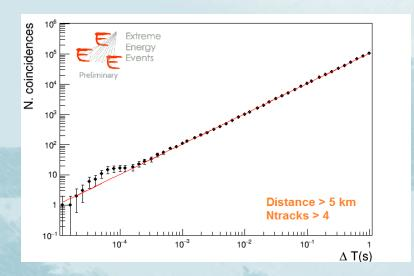
Overall number of coincidences between EEE sites as a function of the time coincidence window, compared with the accidental coincidence background (in red)
