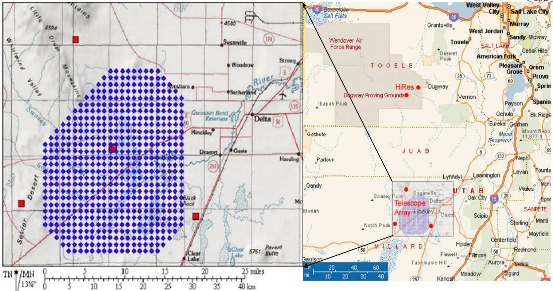
507 scintillation counters surface detector (SD): Area: ~700 km<sup>2</sup>.
