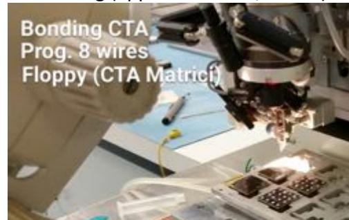
Bonding with 20µm Al/Si wire
