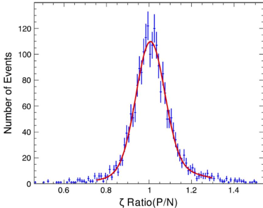
Extended Data Figure 2 | Ratios of the  $\zeta$  values calculated from the  $P$ - and  $N$ -side readout data. The events have deposited energies between 500 GeV and 1 TeV in the BGO calorimeter. The error bars ( $\pm 1\sigma$ ) represent statistical uncertainties. The red line represents a Gaussian fit to the data points. The mean of the ratios is  $1.015 \pm 0.002$  and  $\sigma$  is  $0.110 \pm 0.005$ .
