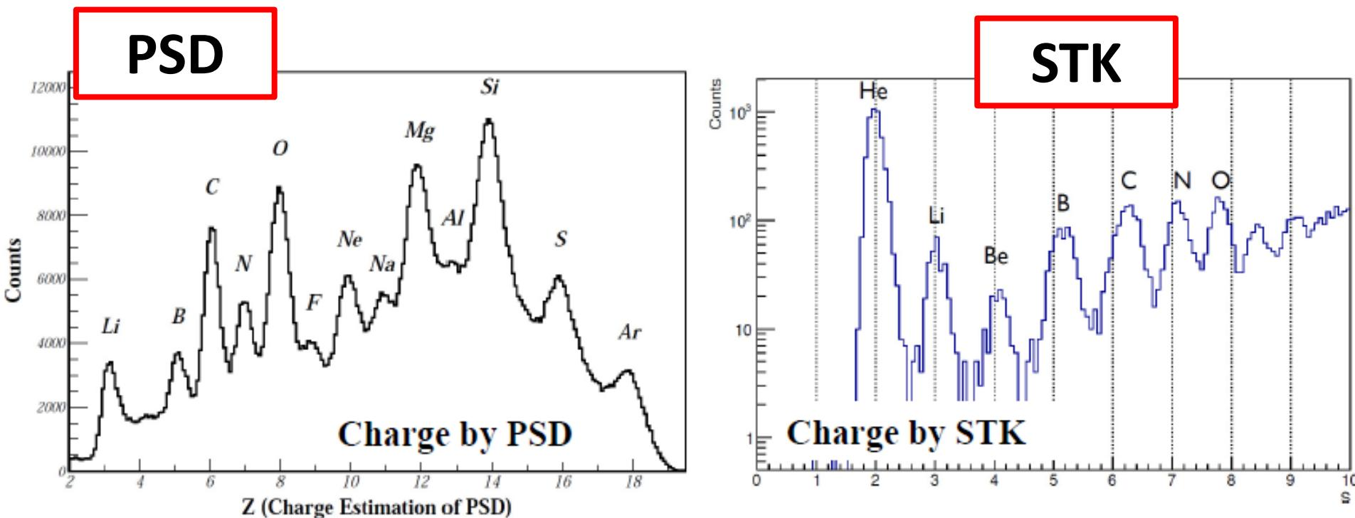
The identification of nuclei is made by using the PSD signal.
