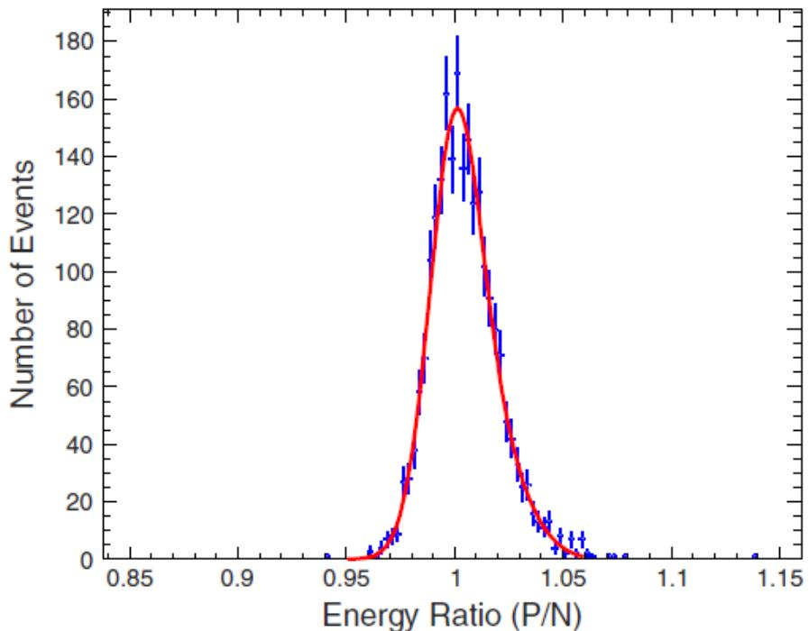
Extended Data Figure 3 | Ratios of the energies reconstructed with the  $P$ - and  $N$ -side readout data. All events have deposited energies between 500 GeV and 1 TeV in the BGO calorimeter. The error bars ( $\pm 1\sigma$ ) represent statistical uncertainties. The red line represents a Gaussian fit to the data, with a mean of  $1.005 \pm 0.005$  and a  $\sigma$  of  $0.016 \pm 0.001$ .
