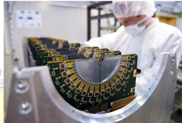
One-half of the VELO under construction
