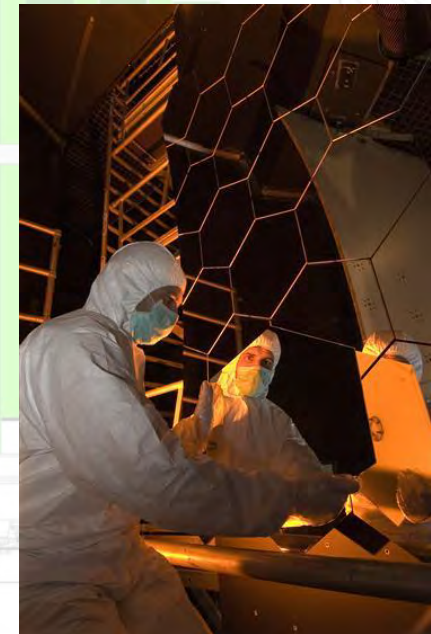
Assembling RICH 2; note the mirrors
