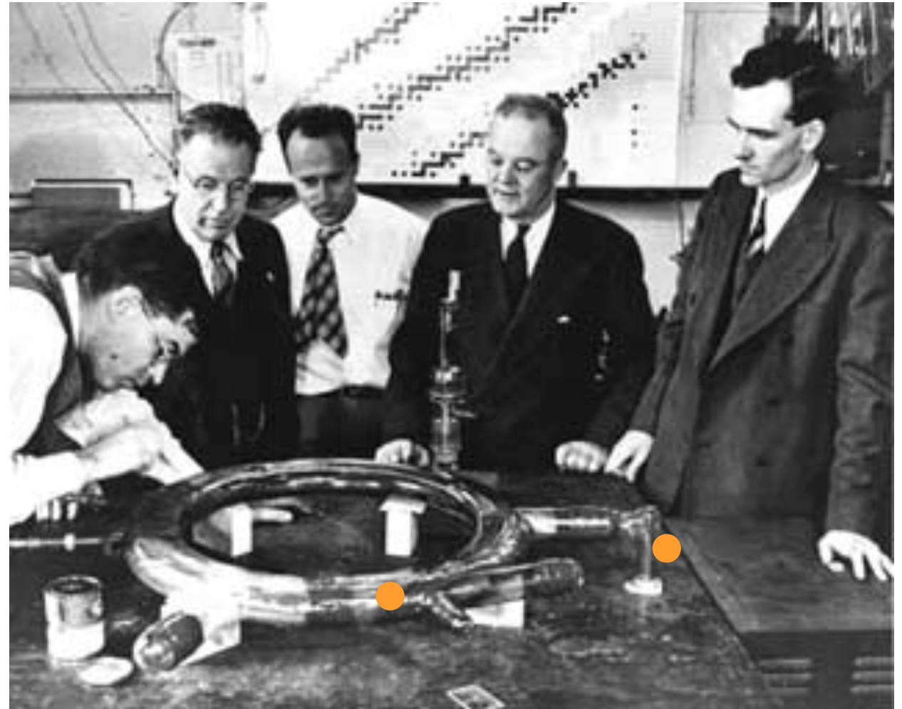
Glass vacuum chamber of the 1947 General Electric Synchrotron Accelerator (70 MeV = 70 million eV). Courtesy BNL and ESRF.
