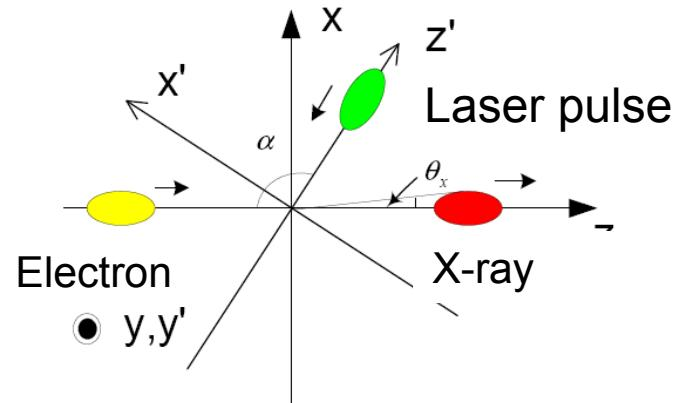
$$\frac{d\sigma}{d\Omega} = r_e^2 \frac{1-\beta^2}{(1-\beta\cos\theta)^2} \left[ 1 - \frac{\sin^2\theta \cos^2 f}{\gamma^2(1-\beta\cos\theta)^2} \right]$$
