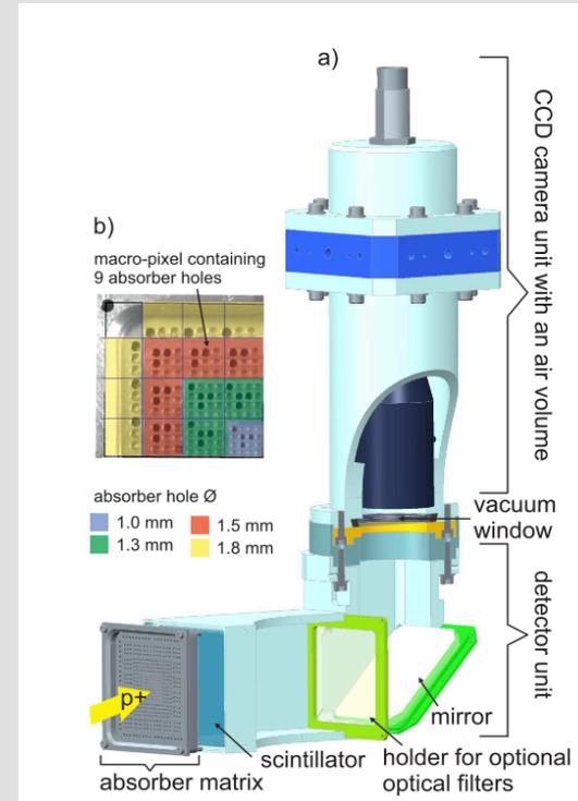
An online, energy-resolving beam profile detector for laser-driven proton beams (2016)
