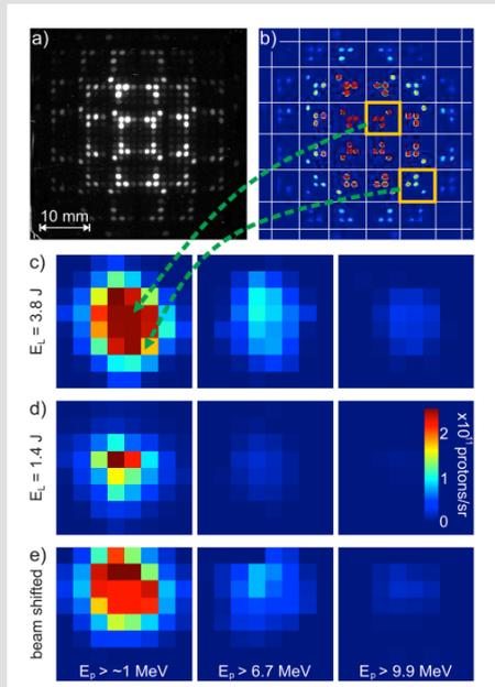
The online detector system resolves the spatial profile of a laser-driven proton beam (4 mm spatial resolution in the central part of the detector) and it can distinguish up to 9 threshold energies.
