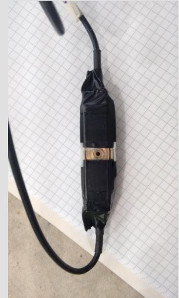
500 micron thickness diamond collimator bore diameter 2 mm
