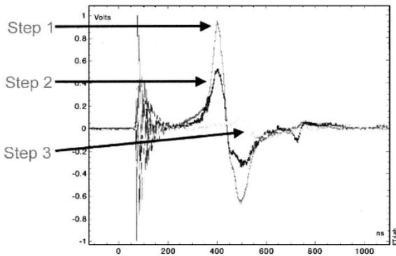
FIG. 5. Single point vs multiple point grounding effect.
