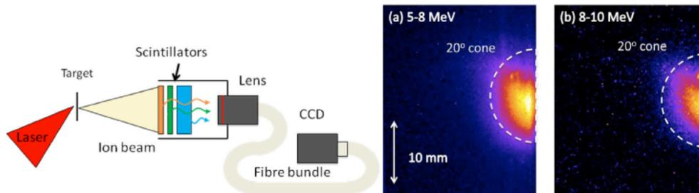
**Figure 6.** (Left) Schematic for a three colour proton beam spatial profiler. Higher energy protons are stopped in the shorter wavelength scintillators located further downstream in the stack. The combined optical signal is collected and relayed to a CCD camera via a fibre optic bundle. (Right) Proton (half) beam profile for two energy windows for a 100 nm Al target irradiated at  $\sim 5 \times 10^{20}$  W/cm<sup>2</sup> with high contrast ( $>10^9$ ).
