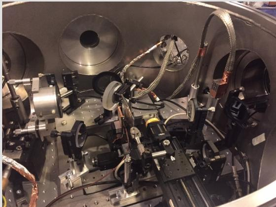
0.7 Tesla permanent magnet inserted to remove unwanted electrons
