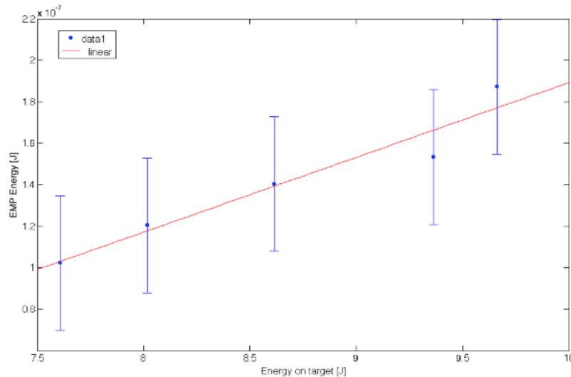
Figure 5.26: EMP energy emission at TARANIS facility as function of Energy released on target (The error bars represent the standard deviations)
