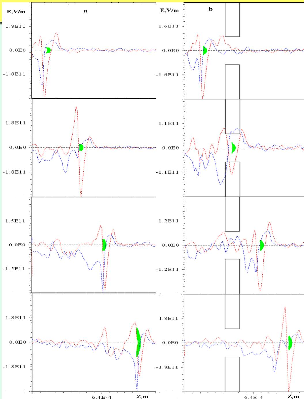
Time depended (time step 400 fs) electron bunch (green dots), longitudinal (red dash line) and transverse (blue dash line) plasma wave electric field distribution in channel at the mean beam radius with (b) and without (a) iris.
