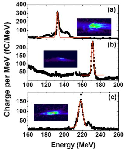
Figure 3: Electron energy spectra showing a bunch (respective false-colour YAG image inset) with (a) central energy = 133 MeV and measured  $\sigma_e/\gamma = 0.8\%$ , (b) central energy = 171 MeV and measured  $\sigma_e/\gamma = 0.7\%$  and (c) central energy = 218 MeV and measured  $\sigma_e/\gamma = 1.1\%$ . Each red curve is a Gaussian fit and the charge in each bunch is  $\sim 0.5$  pC.
