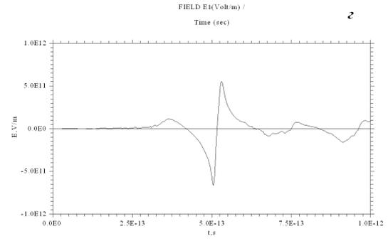
Time depended longitudinal(a) and transverse (b) fields on the axis at the beginning and at the middle (c) of the buncher
