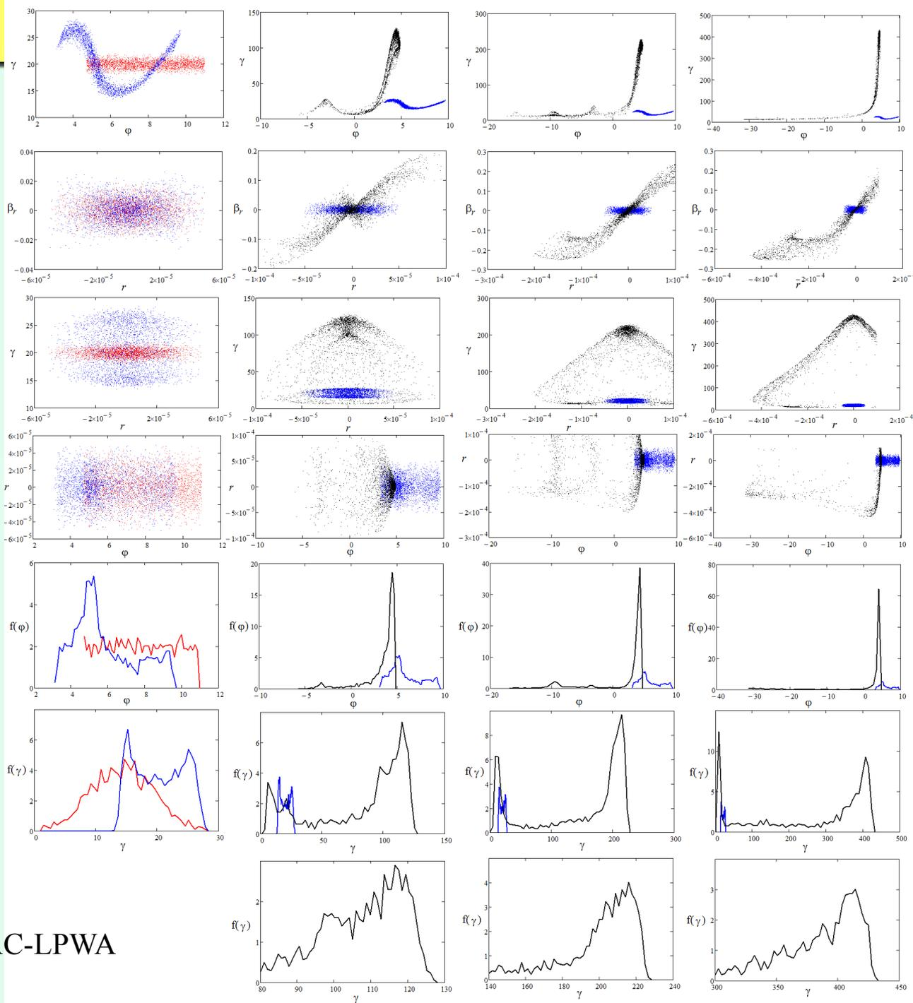
It is clear that the electrons are effectively bunched and captured into acceleration in the main stage. The spectrum is lower than 3 % and decreases with energy. The part of electrons are decapturing of acceleration and part of electrons having maximal energy decreases from 70 % for 120 MeV to 40-45 % for 400 MeV. But such dependence is typical for conventional RF linac also.
