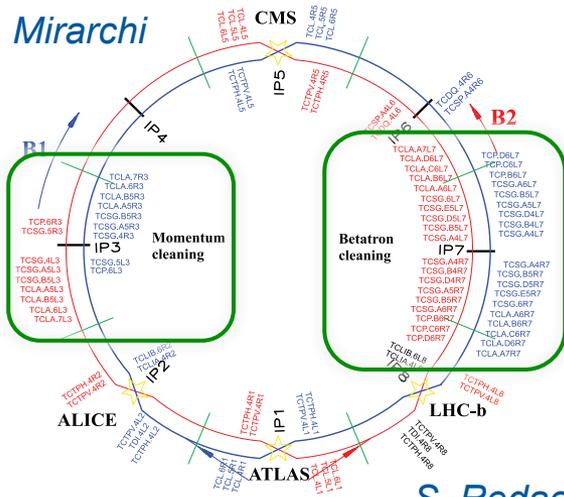
**Multi-stage cleaning with about 50 collimators per beam, two dedicated insertions**
