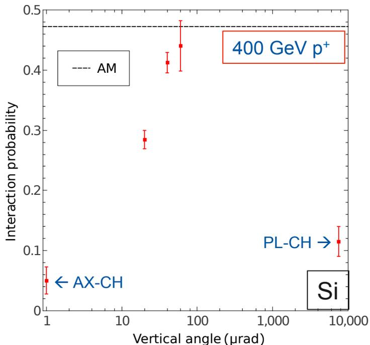
Crystal bending angle  $\Theta=55 \mu\text{rad}$
