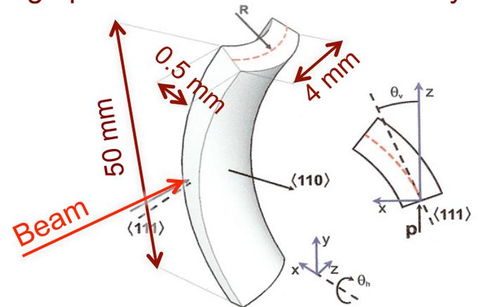
Bending  $50\mu\text{rad}$      $B_{eq} \approx 300 \text{ T @ } 7 \text{ TeV!}$
