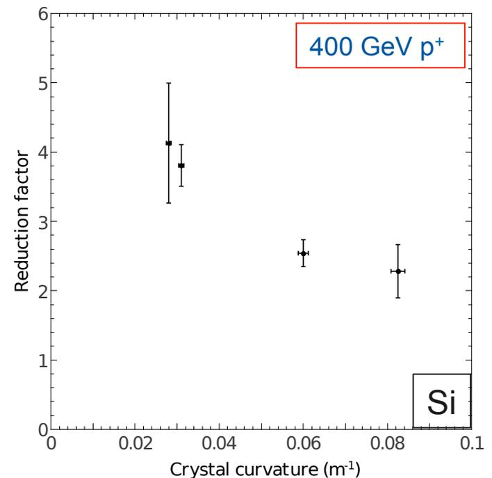
Crystals thickness along the beam: 2 mm
