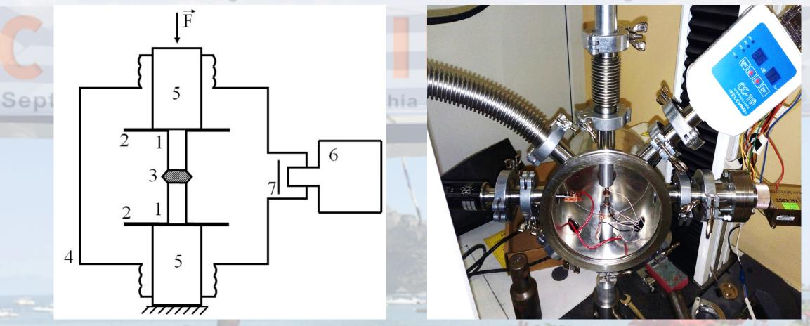
The cylindrical assembly of two piezoelectric ceramics cylinders 1 with copper high-voltage electrode 3 is installed in vacuum chamber 4 between two metal grounded disks 2. The variable force can be applied along the assembly axis through metal cylinders 5. The spectra of X-ray radiation are measured with X-ray detector 6. Mylar foil 7 is installed before the entrance window of the detector.
