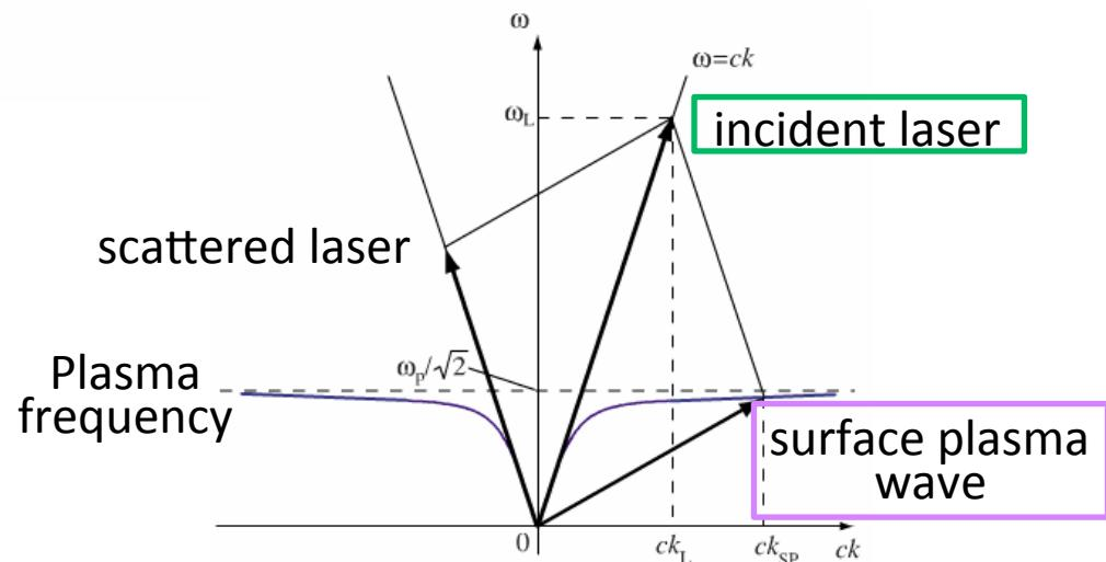
Interference between incident light and surface wave
