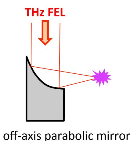
off-axis parabolic mirror
