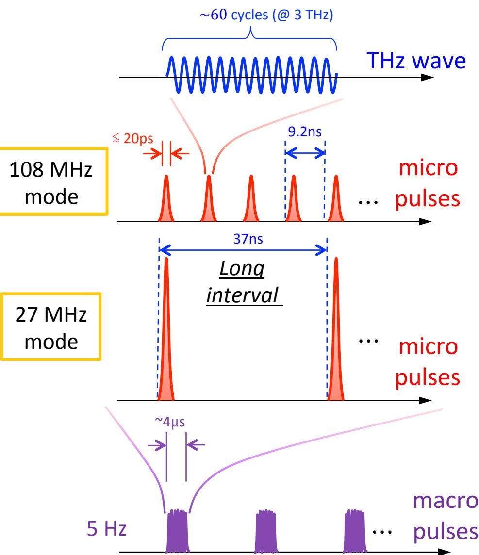
As a result, pulse structures of FEL reflect the e-bunch structures.
