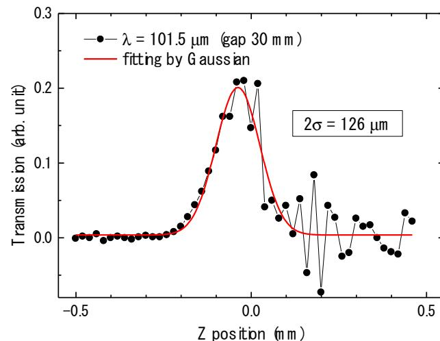
Derivative transmittance (Gauss fit)
