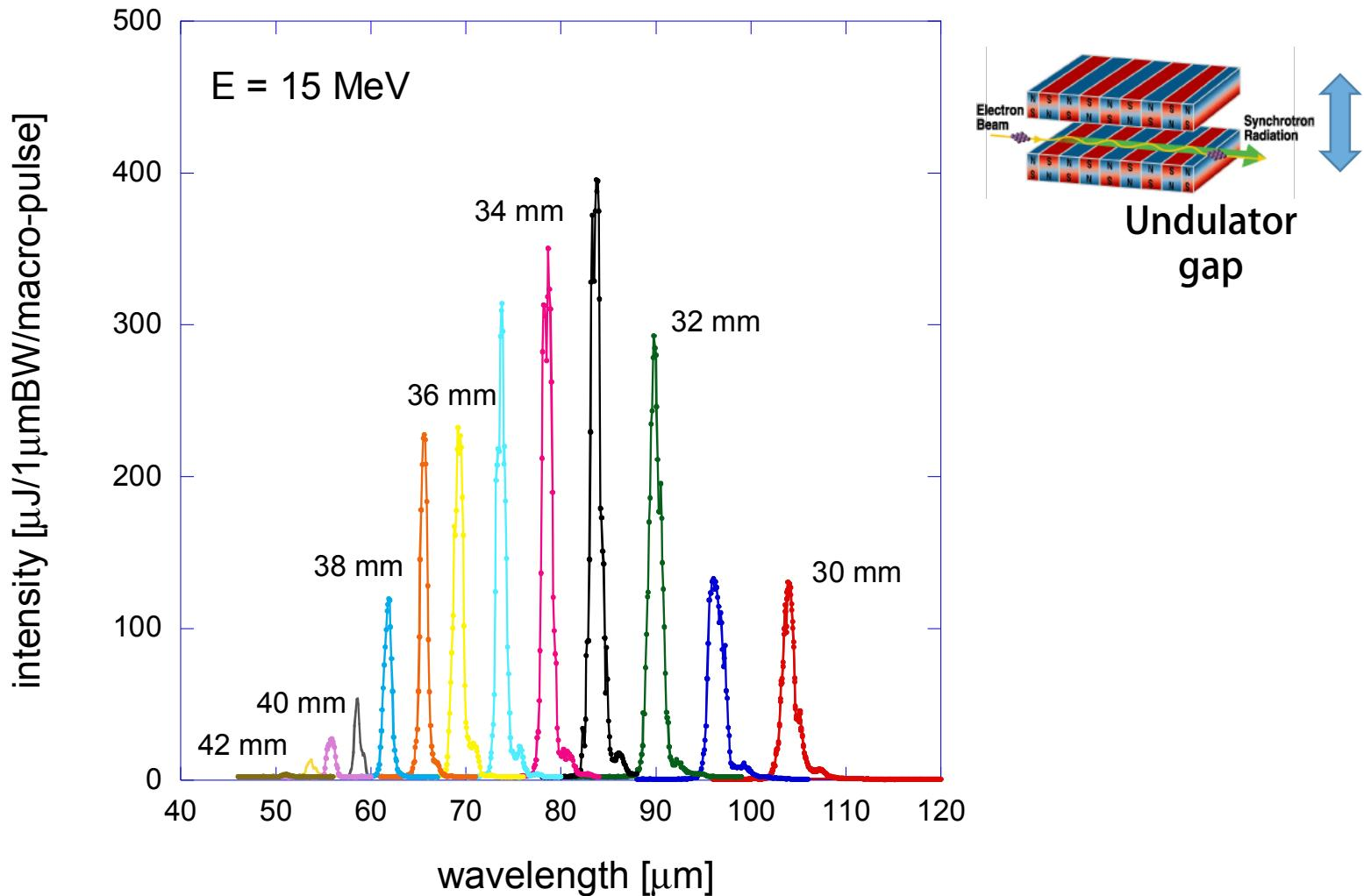
Wavelengths for different undulator gaps
