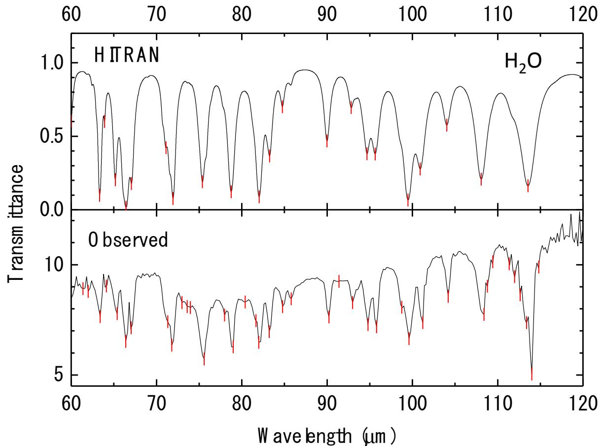
Simulation and measured water vapor absorptions
