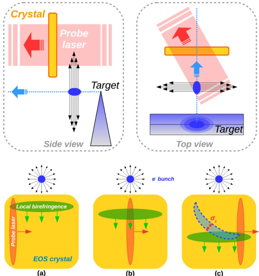
The emitted bunch travels normally to the crystal surface and moves below it while the probe laser crosses the crystal with a non-zero incidence angle.
