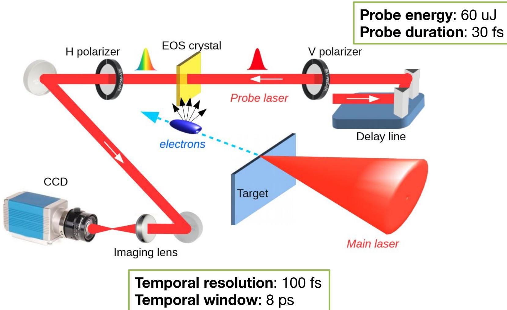
Pompili, R., et al. "Sub-picosecond snapshots of fast electrons from high intensity laser-matter interactions ." Opt.Exp. 24 (2016)
