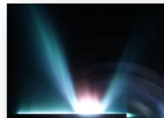
Generation of a monochromatic EUV/SXR radiation from laser-plasma sources
