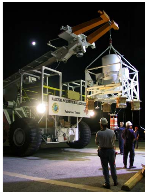
Payload, inside of Pressure Vessel, mounted to GRIS Gondola
