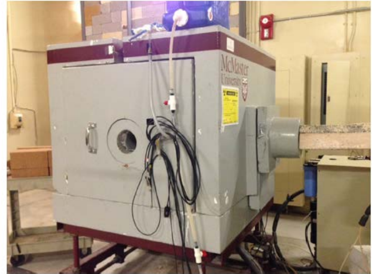
Fig. 1. Irradiation cavity of the Tandemtron accelerator at McMaster University.
