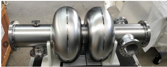
CEPC 650 MHz 2-cell cavity by OTIC
