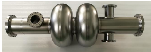
CEPC 650 MHz 2-cell cavity by HERT
