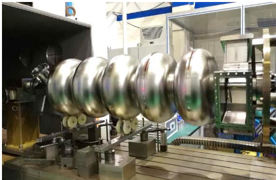
CEPC 650 MHz 5-cell cavity with waveguide HOM coupler by HERT (poster 2AMSP17)
