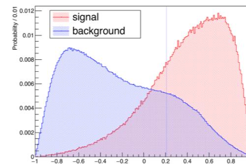
After X cut, BDT Analysis with input variables like Hmass, Zmass KMasses(masses of jet pairs after kinematic fit),  $y_{45}$ , H/Z  $\cos\theta$ , sphericity was applied.
