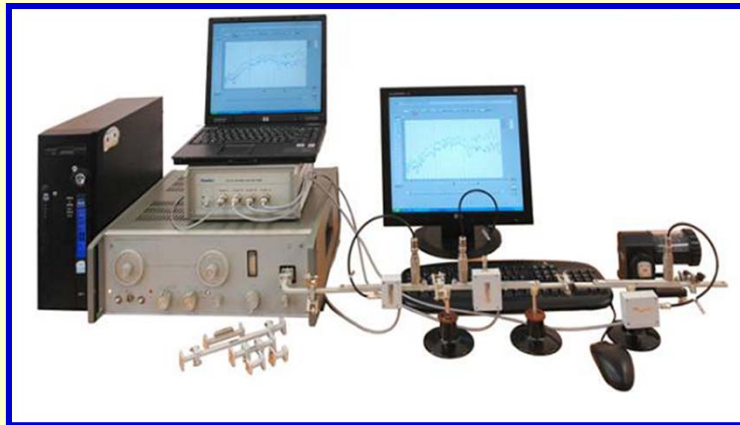
Scalar analyzer R2-408R (VSWR and Transmission Loss Meter R2-408R) 27-37 GHz
