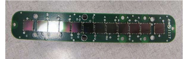
Standard Light Guides are used to instrument 5 of the 6 APA. 12 SiPM of which 3 ganged per readout channel per bar are used for the light detection
