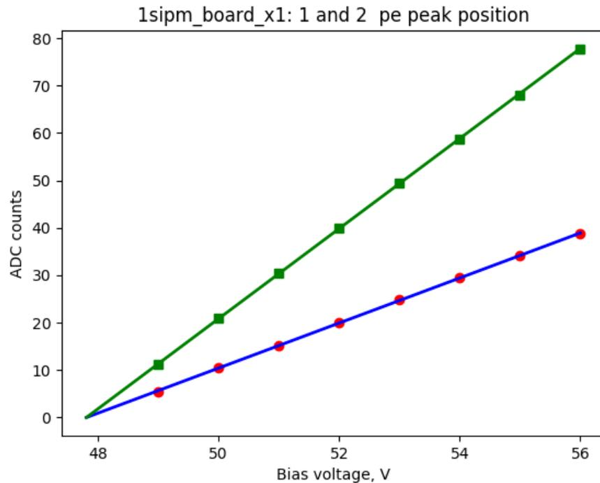
A complete characterization of SiPM Hamamatsu has been made to understand their behavior ( $T = -70\text{C}$ ).
