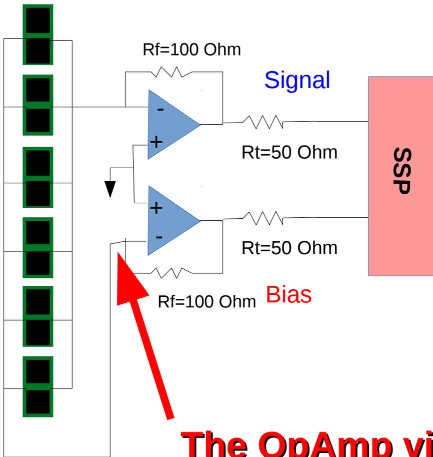
Since the SSP has an amplification stage based on full-differential OpAmps the front-end amplification stage was removed and the buffer was adapted.
