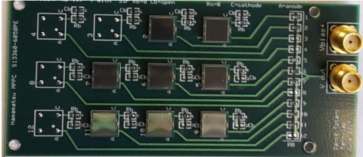
The boards allow for passive ganging of 1 to 12 SiPMs.
