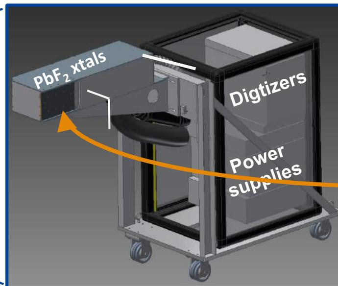
Segmented array of PbF<sub>2</sub> crystals to reduce pileup (was one full block in BNL exp. E821)
