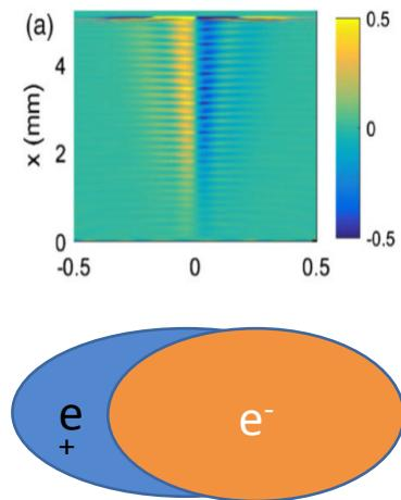
Ultra relativistic **Quasi Neutral beams**, positron bunch embedded into an electron bunch
