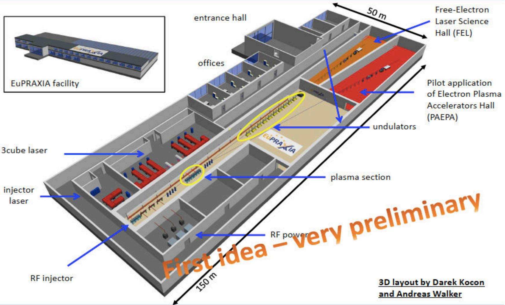
A Free Electron Laser is a device that converts a fraction of the electron kinetic energy into coherent radiation via a collective instability in a long undulator
