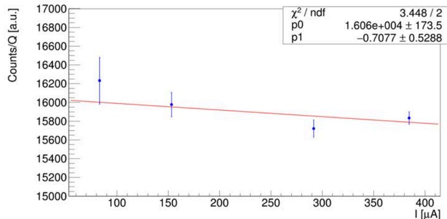
Measurement of the D(p, $\gamma$ )<sup>3</sup>He reaction Yield Vs beam current
