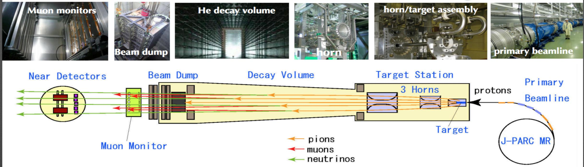
1. Accelerate protons and strike a target producing pions, kaons
