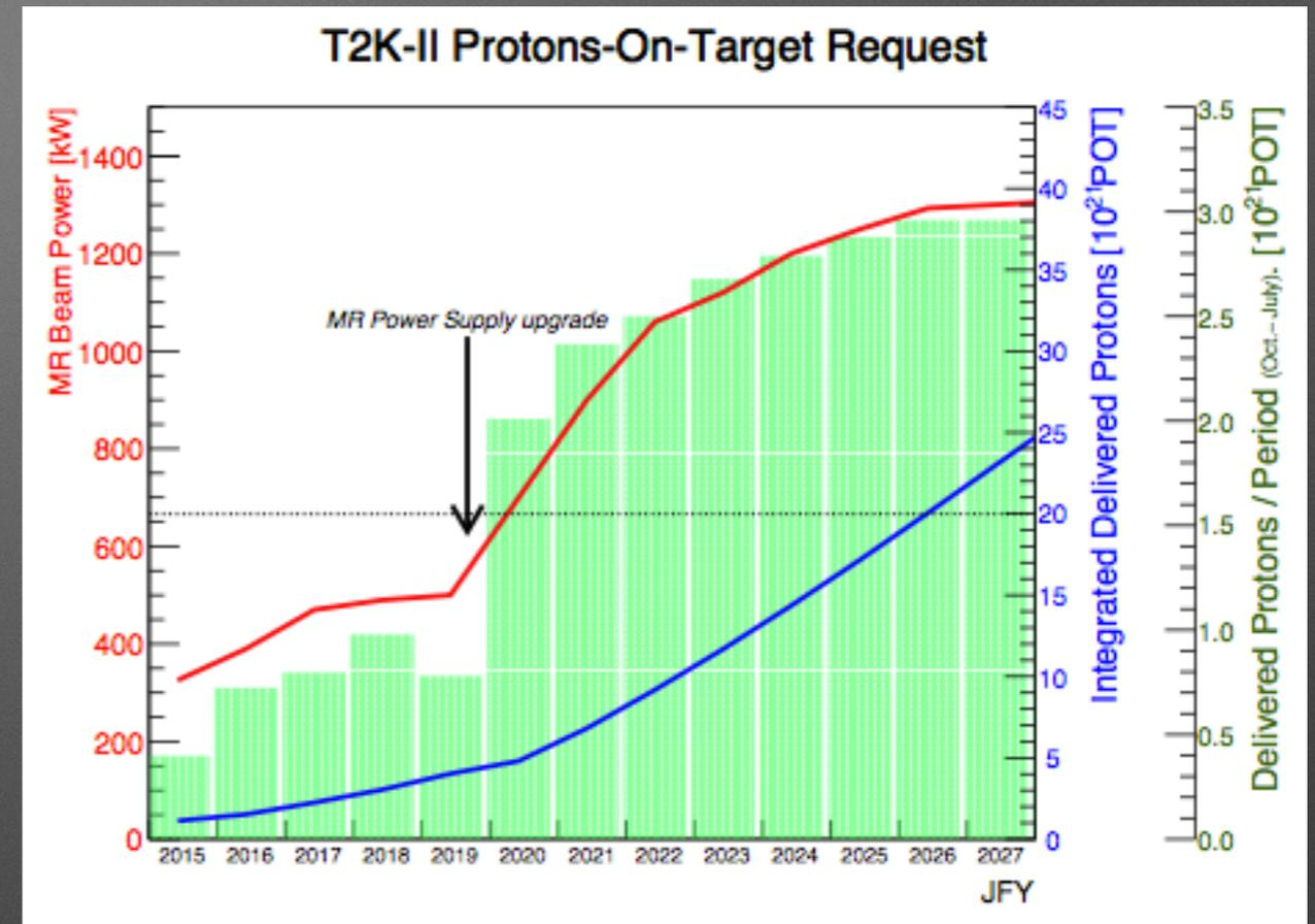
► To reach such statistics (and be ready for HK) we will upgrade the Main Ring power supply to reach 1.3 MW operations
