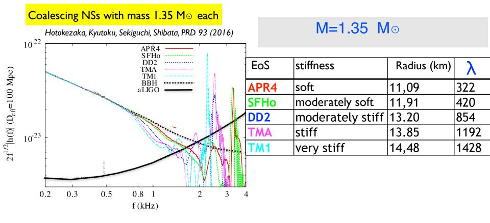
To measure the tidal deformability  $\lambda$  and gain information on the equation of state of matter in the inner core of the stars we need detectors more sensitive at frequencies larger than ~ 500-700 Hz
