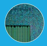
More complex logics have been design with automatic tools based on standard cells (synthesis, place & route)
