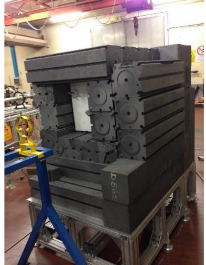
Moderator, low power@CN accelerator at INFN
