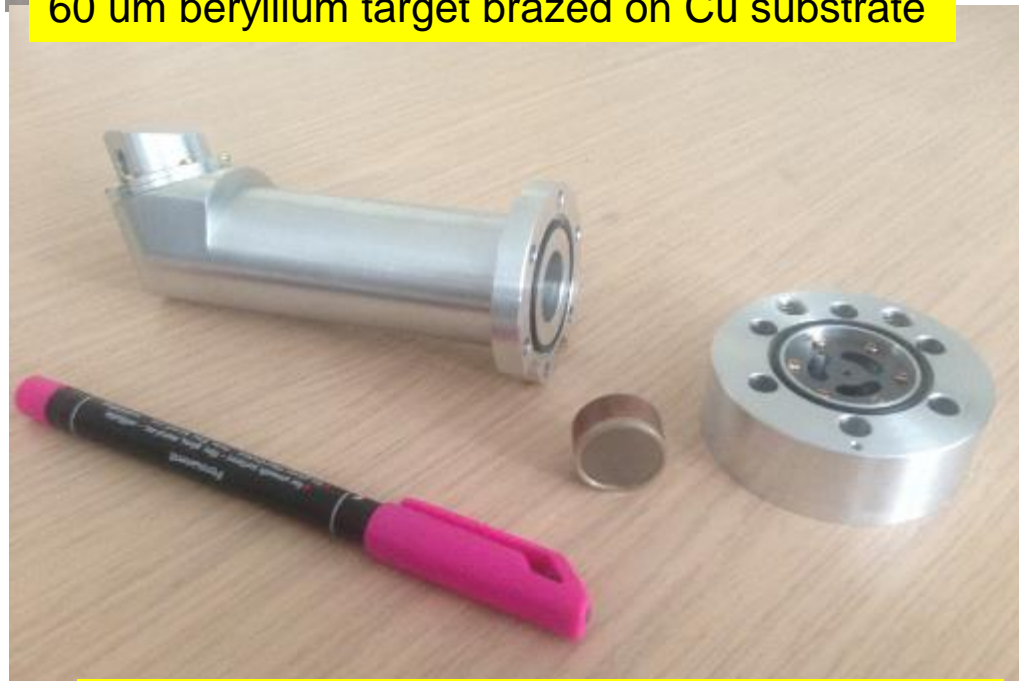
Target, holder and beam collimator (low power)
