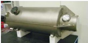
High beta cavity prototype with its helium tank
