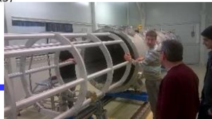
Blank assembly of the spaceframe inside the vacuum tank
