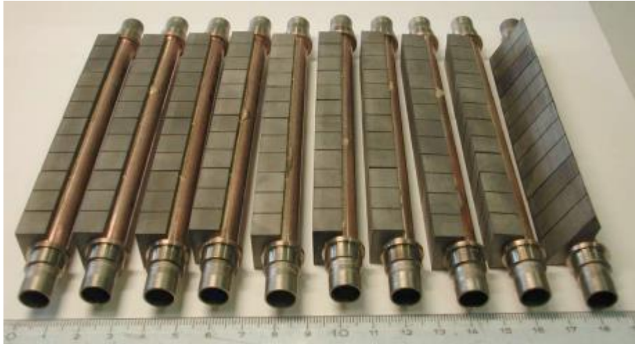
1. Be tile brazed cooling pipes
