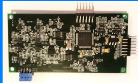
40 independent acquisition channels operating in two modes (slow calibration and fast counting)
