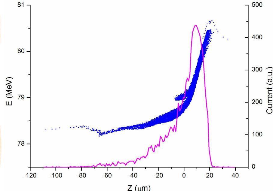
$$I_z \approx 36 \text{ } \mu\text{m} \text{ (FWHM.)} \quad \sigma_z \approx 28 \text{ } \mu\text{m} \text{ (r.m.s.)}$$
