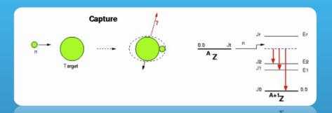
Capture reactions are measured by detecting  $\gamma$ -rays emitted in the deexcitation process
