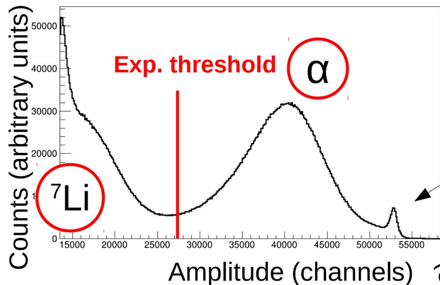
~6% of lithium produced is in the ground state with more kinetic energy available for the  $\alpha$
