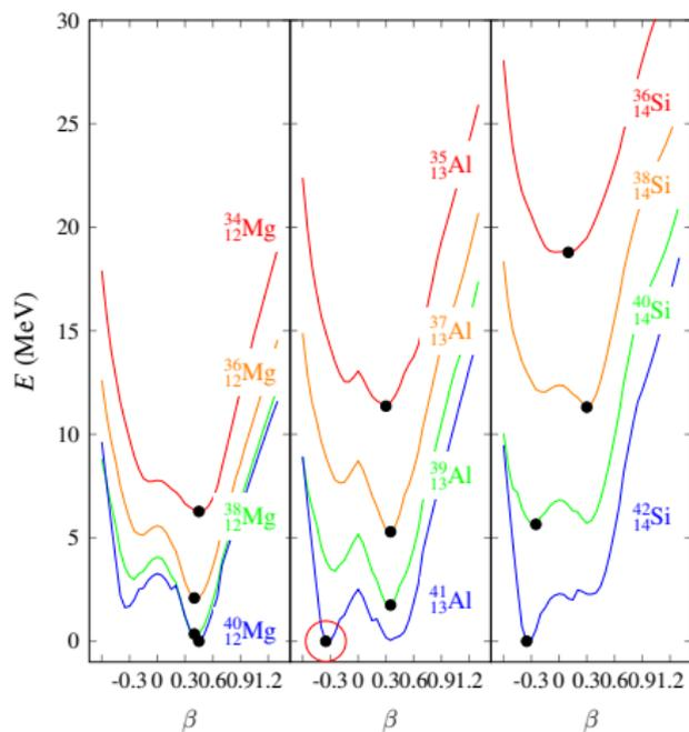
Hartree-Fock-Bogoliubov mean-field calculated energy surfaces with the D1S Gogny effective interaction Berger, Girod, and Gogny 1991 from the AME00 database Hilaire and Girod 2007. The surfaces of Mg, Al, Si are offset for visualization.
