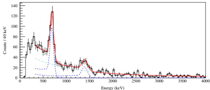
Fit of  $^{34}\text{Mg}(^9\text{Be,X})^{32}\text{Ne}$  doppler reconstructed  $\gamma$ -ray energy spectrum,  $m_\gamma \leq 3$ , and with add-back
