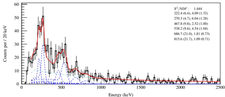
Fit of  $^{41}\text{Al}(\text{C}/\text{C}_2\text{H}_4, \text{X})^{40}\text{Al}$  doppler reconstructed  $\gamma$ -ray energy spectrum,  $m_\gamma \leq 5$ , and with add-back
