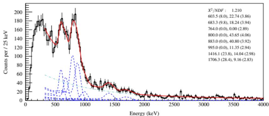
Fit of  $^{40}\text{Al}(\text{C}/\text{C}_2\text{H}_4, \text{X})^{39}\text{Al}$  doppler reconstructed  $\gamma$ -ray energy spectrum,  $m_\gamma \leq 5$ , and with add-back
