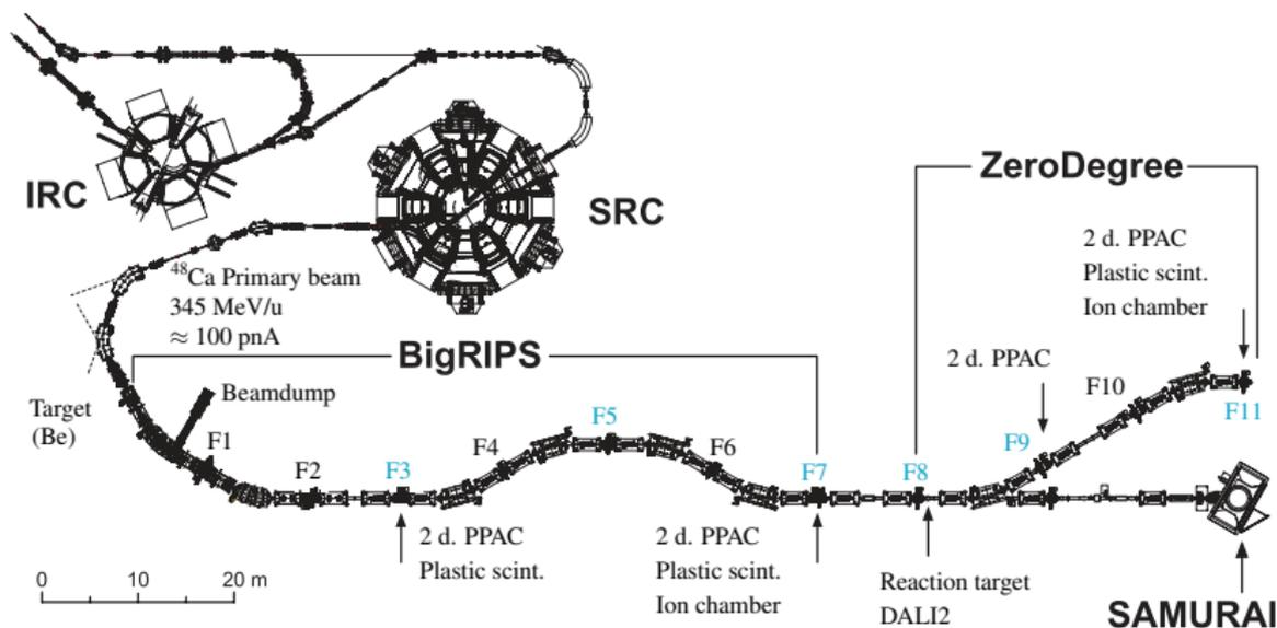
Overview of the IRC, SRC accelerators and the BigRIPS separator and ZeroDegree spectrometer. Image from Kubo et al. 2012.
