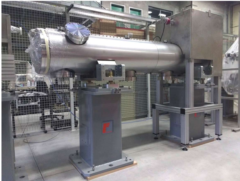
A Compton Spectrometer to monitor the ELI-NP beam energy R. Borgheresi et al. PM2018 -14th Pisa Meeting on Advanced Detectors,NIM-A proceedings (in review)
