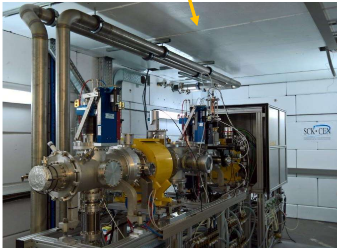
ECR source: Pantechnik LEBT: coll. LPSC Grenoble, IPHC Strasbourg (MARISA, MYRTE), installed at SCK•CEN vault at CRC/UCL for commissioning
