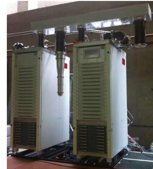
RFQ Solid State amplifier manufactured by IBA (coll. In MYRTE project), installed, under tests
