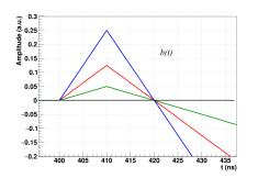
$$\sigma_{ARC} = \frac{t_{rise}}{\text{SNR}} \frac{\sqrt{1+f^2}}{1-f}$$
