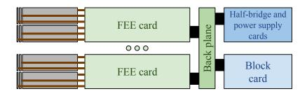
8 FEE cards are connected to a block card via a back plane.
