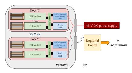
up to 36 block cards are connected to a regional board via a full duplex 3 Gb/s optical link
