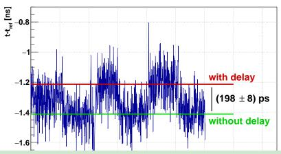
Expected  $(t - t_{ref})_{del} - (t - t_{ref})_0 = t_{del} \simeq 207 \, \mathrm{ps}$
