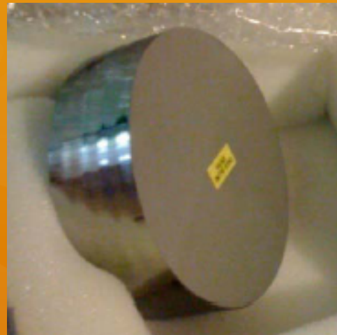
SuprCDMS HP Ge detectors are fabricated in 100 class clean room.
