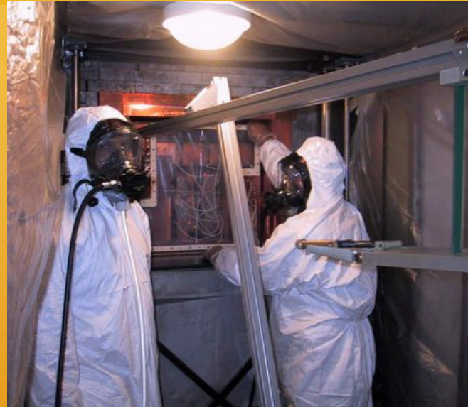
DAMA shielding cage and detectors: they are protected by overpressure of High Purity N 2 gas
