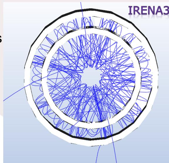
Without magnet ! Space charge → repelling the electrons.
