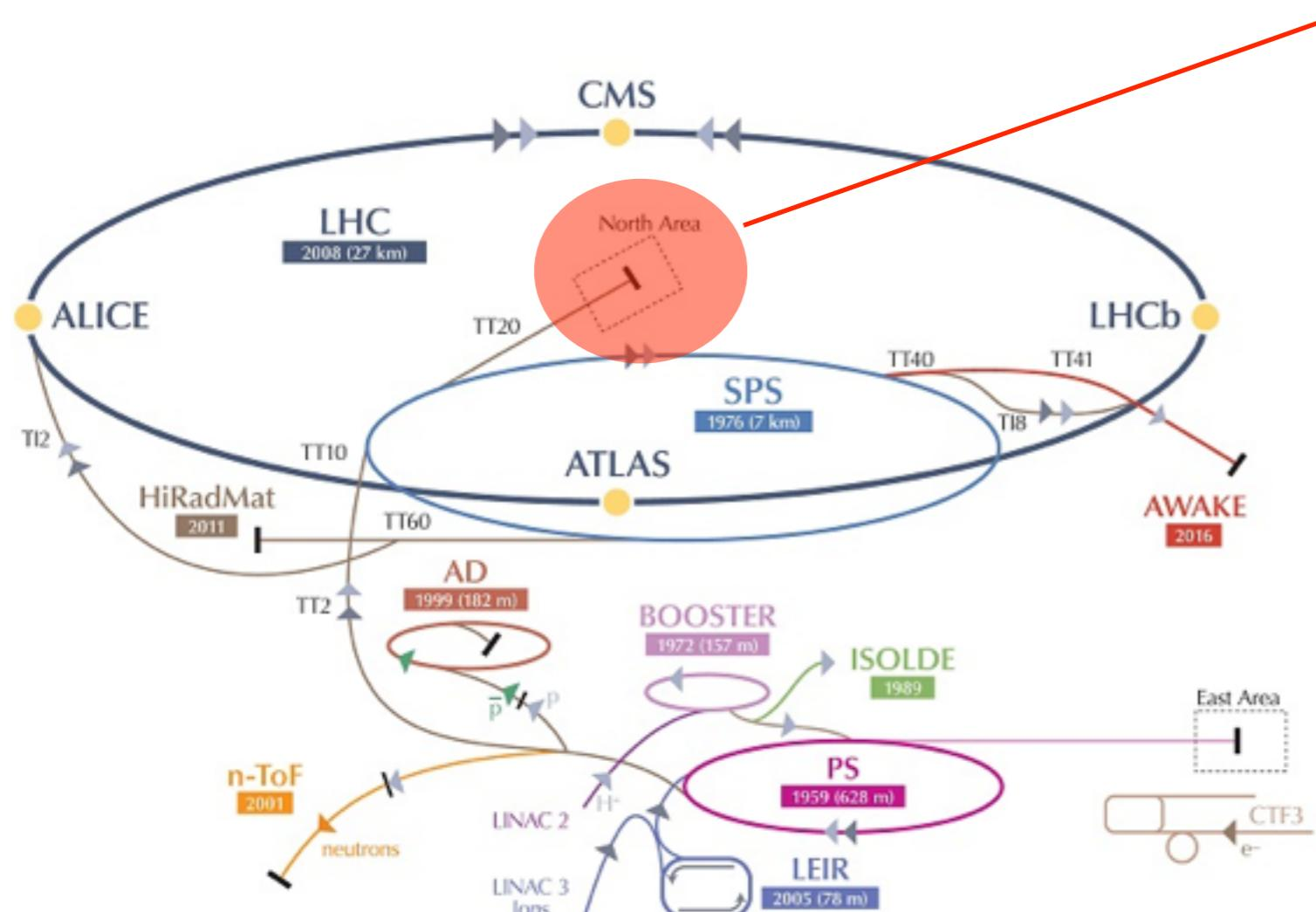
In the North Area the SpS extraction line is providing a secondary charged hadron beam
