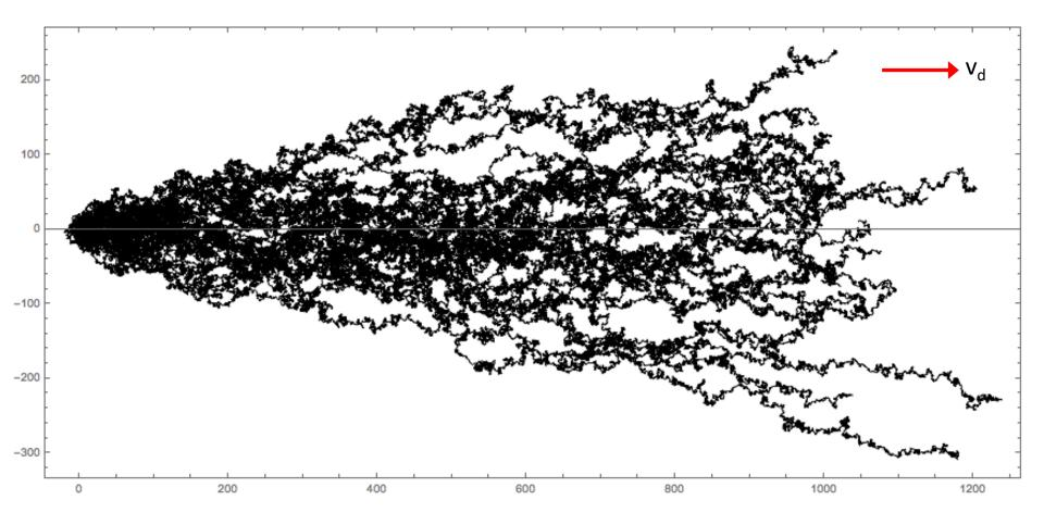
The diffusion coefficient of electrons in Cu associated with this random motion can be computed from the Einstein formula
