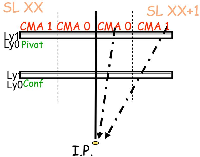
RPC spatial correlation between trigger strip (Pivot) and confirm strip (LowPt) in phi view for a programmed trigger road in cosmics data
